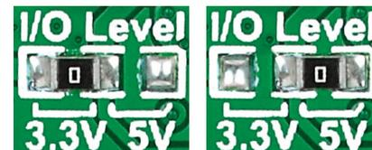
There is one zero-ohm SMD jumper **J1** used to select whether 3.3V or 5V I/O voltage level is used. Jumper **J1** is soldered in 3.3V position by default.
