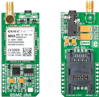
GSM2 Click™ is an accessory board in **mikroBUS™** form factor. It's a compact and easy solution for adding GSM module to your design. It features **Quectel M95** GSM module, audio connector, SIM card socket as well as SMA antenna connector. GSM2 Click™ communicates with target board microcontroller via **mikroBUS™** UART (Tx, Rx), PWM, INT, AN, RST and CS lines. The board is designed to use 3.3V and 5V I/O voltage levels. LED diode (GREEN) indicates the presence of power supply.
